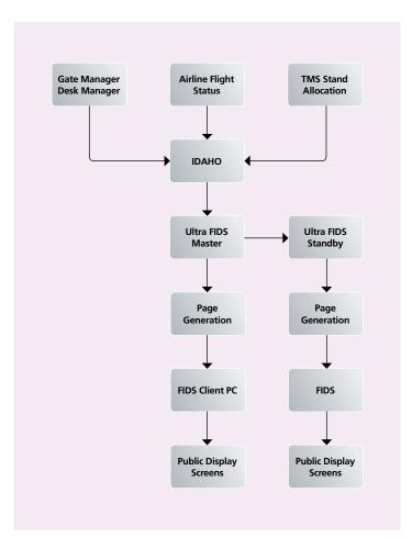
There are currently two separate FIDS applications in use at LHR, FIDS T1-T4 and FIDS T5. Oracle Database software is installed on each server although the actual database storage is on the SAN.
